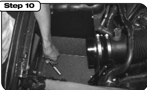
Step 10 Using the 4 bolts from the stock mounting plate fasten the aFe intake housing on the chassis.
