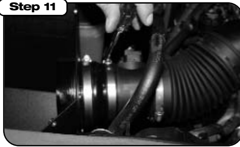
Step 11 Using the reducer coupler, insert and clamp the MAF sensor onto the aFe housing.
