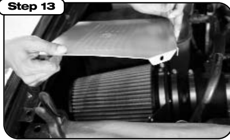
Step 13 Install the housing cover and fasten using three button head screws.
