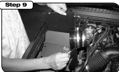
Step 9 With the filter adapter and reducer coupler installed, lower the aFe intake housing into the engine compartment.
