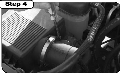
Step 4 Loosen the clamp attaching the MAF sensor to the intake housing.
