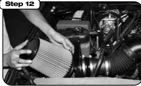
Step 12 Insert and fasten the aFe air filter.
