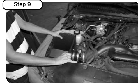
Place the rubber trim seal along edges of the housing.. Bolt the housing to the engine bay using the factor bolts removed in step 6. If installing stage 1 kit re-connect factory tube to MAF sensor.
