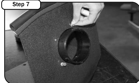
Place the air filter adapter inside the housing. Secure the adapter with the secured bolts and washers.
