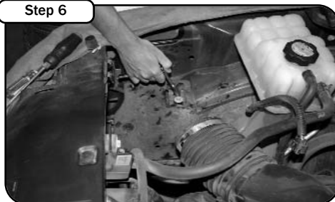
Remove the four 10mm bolts that secure the air box base to the chassis. Save bolts for later use. Remove air box tray out of vehicle.
