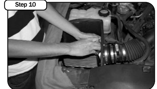
Install intake filter into housing. Re-connect the MAF sensor. Complete stage 1 system installed. Your installation is now complete. Make sure you tighten all clamps and check all electrical connections. Re check periodically. Continue onto steps 11-13 to install stage 2.
