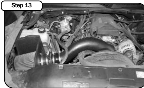
Place enclosed CARB EO sticker on a clean/smooth surface on or near the intake system. EO identification label is required in passing the Smog Check inspection. Make sure all hoses and clamps are tight and that all electrical components are secure.
