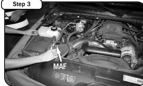
Disconnect negative terminal from battery. Remove the four Phillips screws securing the top of the air box. Disconnect the MAF sensor.
