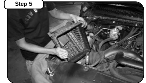
Grab the lower portion of the air box. lift up and out. The box is secured with rubber gromets.
