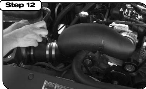
Step 12 Attach the aFe intake tube onto the MAF and throttle body. Secure the clamps when properly positioned. Connect the supplied crankcase breather hose to the intake tube.
