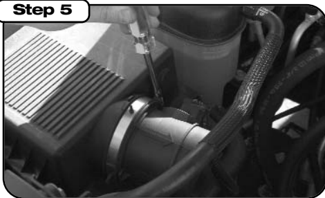
Step 5 Loosen the clamp attaching the MAF sensor to the intake housing. Remove the MAF sensor.
