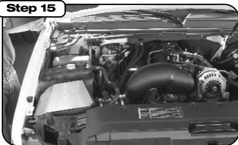
Step 15 Your installation is now complete. Make sure to tighten all clamps and check all electrical connections. Re-check periodically.
