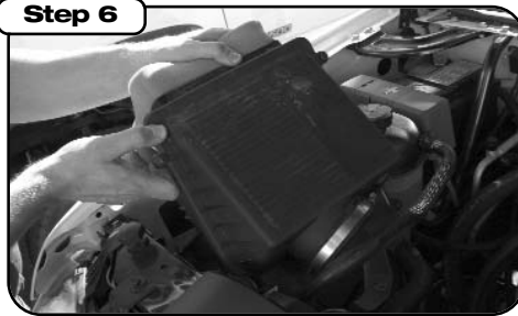
Step 6 Lift up and out to remove the stock air box.
