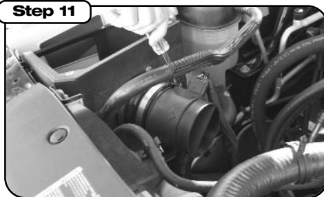
Step 11 Using the reducer coupler, clamp the MAF sensor onto the aFe housing. If this is a flex-fuel vehicle, use second reducer coupler between sensor and intake tube.
